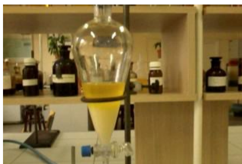
Figure 3. The partition of carotenoids in carrot sample
