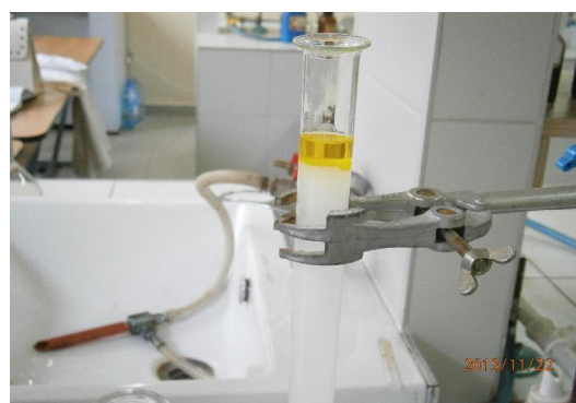
Figure 4. Chromatographic separation in open column
